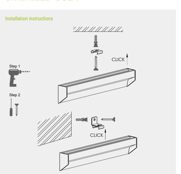
When fitting the clamp, make sure that it can still be turned slightly, otherwise it can cause cracking noises due to thermal expansion.
