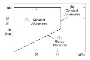
Typical LED power supply I-V curve
