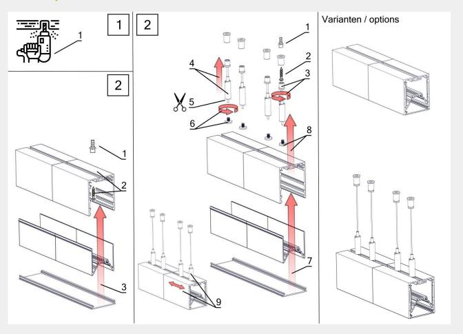
It is absolutely essential to earth the outer channel!During disassembly, use a screwdriver to pull down the inner profiles at the holes provided for this purpose.
